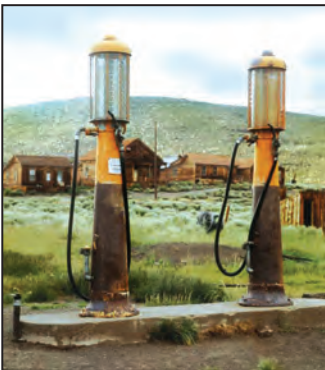
Photo 1.1 In the early days, gas was pumped out of the ground into a clear glass cylinder that showed what you were getting, including if the gas was dirty (a big problem at that time). From there, it flowed by gravity down the hose into the car. Only the calibration marks on the cylinder express true visual information sharing—for viewing and measuring the gas as it flows out.
