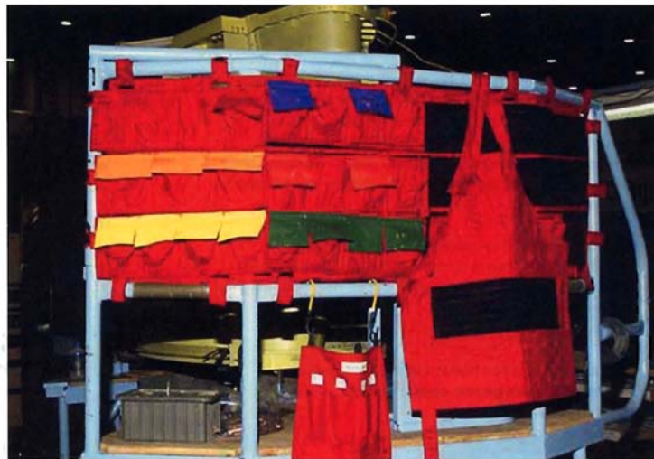
A Visual workplace inspires creativity: The "apron" above was the idea of an assembler at Lockheed Martin Aerospace who noticed how frequently he and coworkers could not find tools that they needed. He crafted the big red apron, and added Velcro and color-coding to make storing and locating tools a snap.
